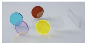
Examples of various colors by changing dopant ions in YAG
